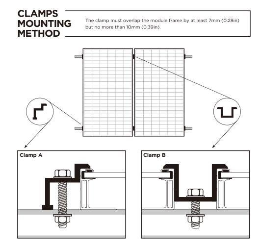
Secure the module in each mounting location with an M8 bolt and a flat washer, spring washer and nut as shown in Figure 1 and tighten to a torque of 16-20 N.m(140-180lbf.in.).
