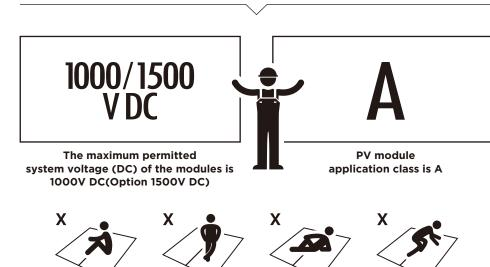
\* When Module exposed to sunshine or other lights, it can produce DC, in this case it may cause electric shock hazard if touch electrical parts.
